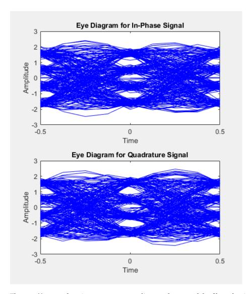
The eyediagram function creates an eye diagram for part of the filtered noiseless signal. This diagram illustrates the effect of the pulse shaping. Note that the signal shows significant intersymbol interference (ISI) because the filter is a square-root raised cosine filter, not a full raised cosine filter.
