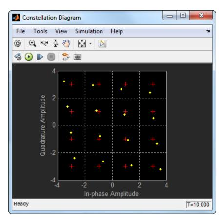
You can see that I/Q amplitude and phase imbalance has shifted the constellation diagram so that each symbol is not exactly equal to its reference symbol (shown in red). Change the I/Q Imbalance block to see the effects of differing imbalances on the constellation diagram.
