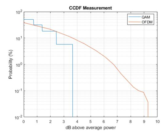
Compare the PAPR values for the QAM modulated and OFDM modulated signals.
